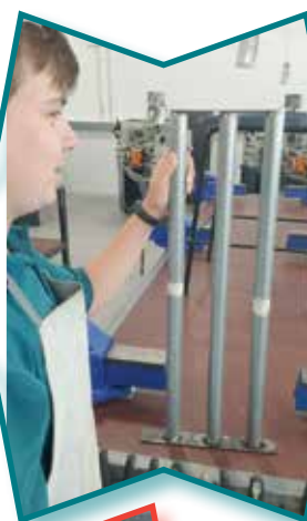
Back yard cricket stumps being constructed in Mr Brittains Year 9 Metal work class. A variety of skills are used ranging from welding, grinding and cutting.
