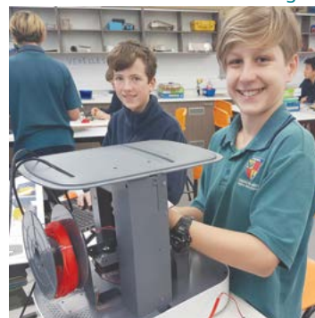
Students are working on building a 3D printer from a kit
